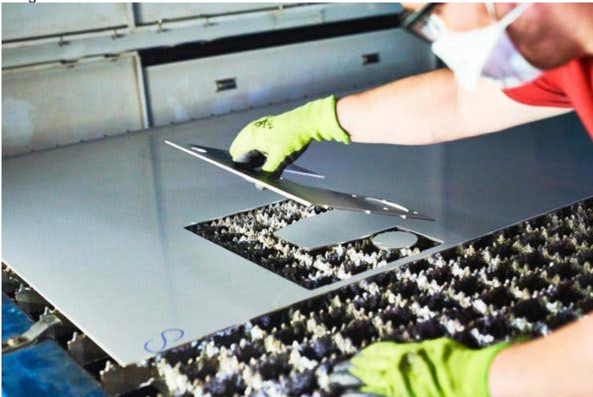
*A steel sheet being cut for the top chassis of a ventilator. Gabby Jones for The New York Times*
